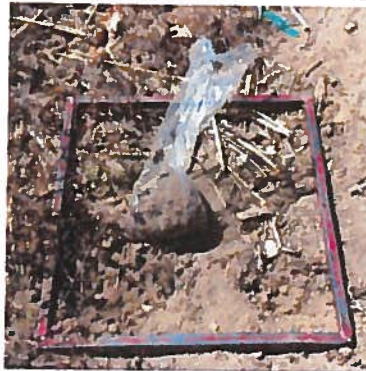
Place the soil sample in the plastic bag and tie the top of the bag so that no soil is lost and it is safe for transporting
