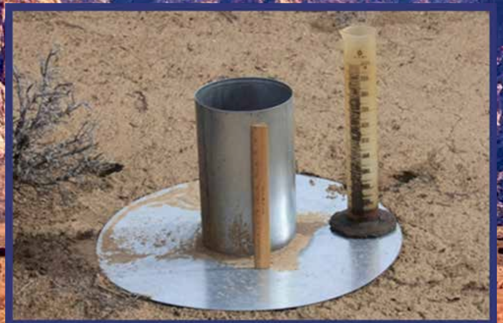
Photo 1: Portable precipitation gauge with ruler and beaker utilized by USDA ARS to measure precipitation on rangelands.
