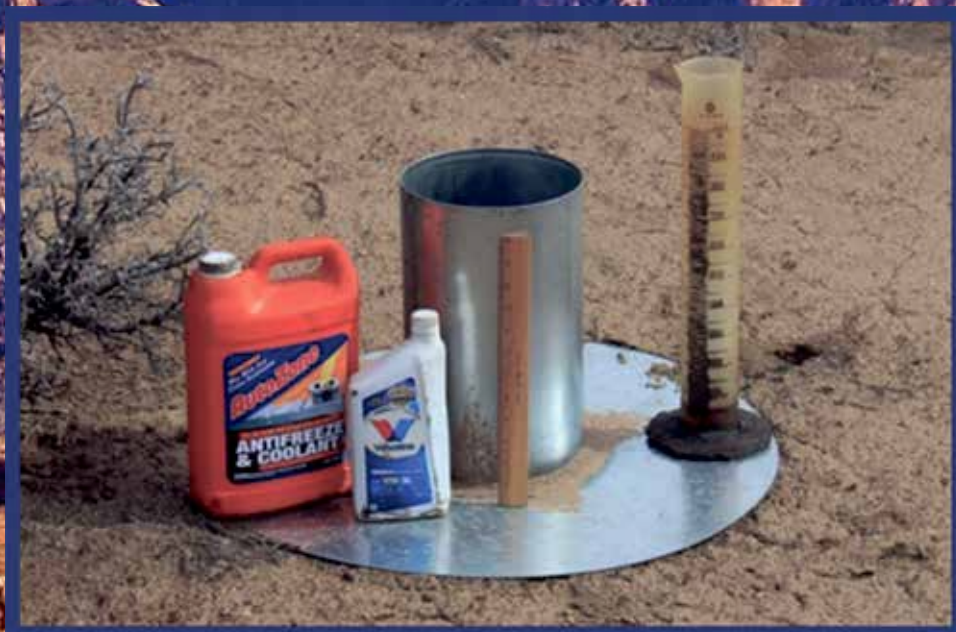
Photo 2: Portable precipitation gauge with anti-freeze and motor oil utilized with appropriate mixes to fit seasonal changes. Beaker used to measure mL of fluid.
