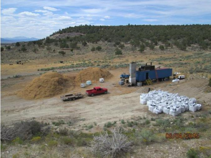
**Photo 2:** Shows one of ten Nevada Division of Forestry mobile kilns in White River. A finished pile of biochar is shown on the left with an active kiln on the right. Note the difference between the residual slash in the foreground versus the background, as well as the contrast between the treatment area, and the untreated area in the background.
