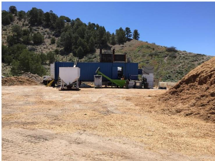
**Photo 1a:** Shows Amaron Energy's rotary kiln in Eureka. The kiln is housed inside the large shipping container, and is fed by the white chip feed bin and conveyor on the left. Finished biochar is emptied from the kiln into the green finished char bin and conveyor in the center, cooled with a water spray, and dumped into super sacks for storage and transportation. The equipment to the right of the finished char bin includes an incinerator and waste oil container.
